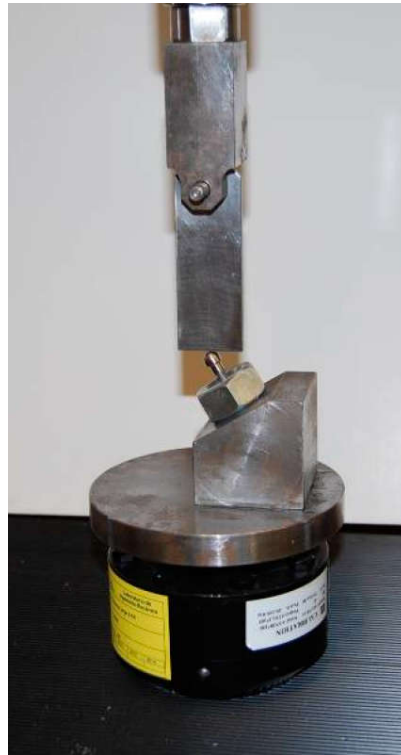
Figure 3. Load cell over the sample in the testing machine.
